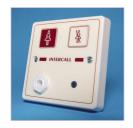
L622 standard call point – a call point is needed for every individual call location on the system. Every L622 unit features five levels of call, multi-colour re-assurance LED alerts and a 'call follower' sounder. The jack socket accepts inputs from a wide range of triggering devices such as pear leads, pressure mats and portable radio triggers.
