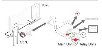
The S37L Wristband Transmitter with Locating function is built to interact with the following devices:
